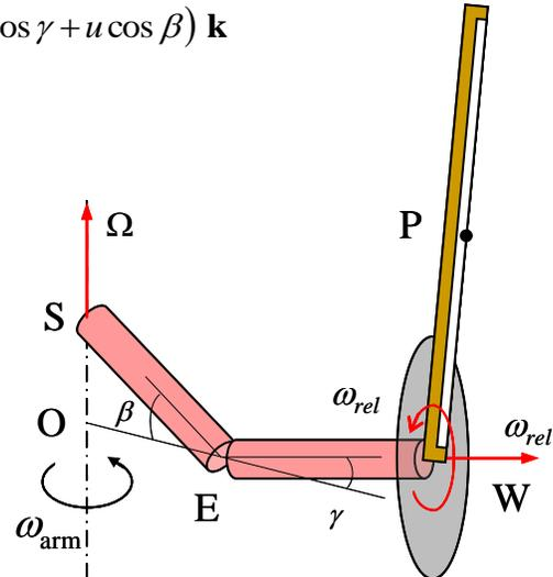
The coordinate system is fixed with respect to the arm so the angular velocity of the bow with respect to the coordinate system is:
