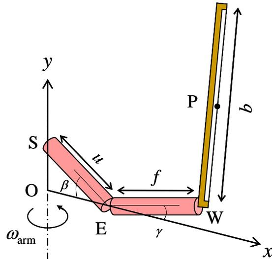
We can establish a coordinate system which is fixed relative to the arm with the  $x$ -axis in the plane SEW and the  $y$ -axis co-incident with the axis of rotation, i.e with an origin at O. So the angular velocity of the arm,  $\omega$  and of the coordinate system,  $\Omega$  are equal and  $\omega_{arm} = \Omega = \omega_0 \mathbf{j}$ . Thus, we can consider the position vector of W relative to O:
