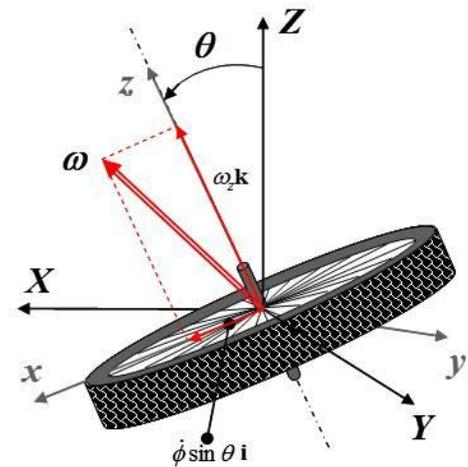
The angular velocity of the wheel is the vector sum of rate of spin about the local z-axis,  $\phi$ ; nutation about the global Y-axis,  $\theta$  and precession about the global Z-axis,  $\psi$ :
