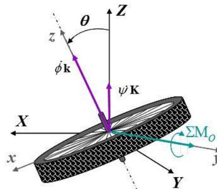
This is the couple that must be applied to maintain the steady precession, i.e.  $\dot{\theta} = \dot{\psi} = \ddot{\phi} = 0$  assuming that the center of gravity of the wheel is fixed in space ( $\Sigma F=0$ ).
