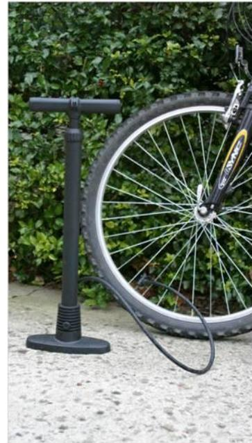
$$\text{Circumferential stress, } \sigma_1 = \frac{pr}{t} = \frac{(6 \times 10^5) \times 0.02}{1.25 \times 10^{-3}} = 9.6 \times 10^6 \text{ N/m}^2$$
