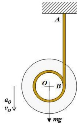
The center of mass of a yoyo will fall at a constant acceleration due to gravity:  $a_o = 9.81 \text{ m/s}^2$  so at the end of its 1.15m string it will have achieved a velocity given by:
